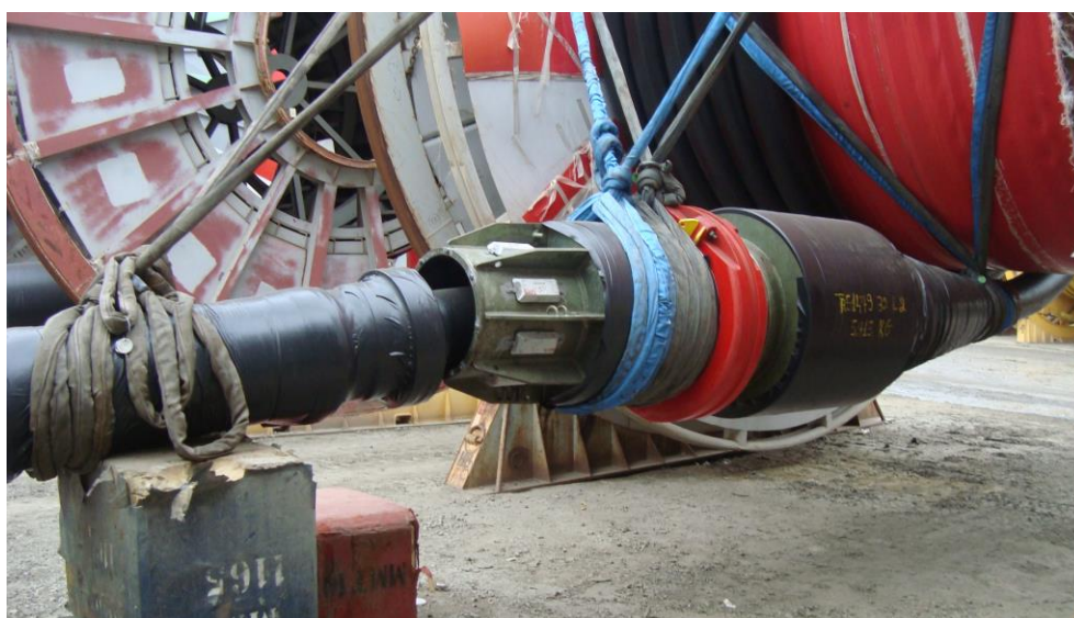
Figure1. Riser Terminal - In preparation for pigging process of removing incrustations
