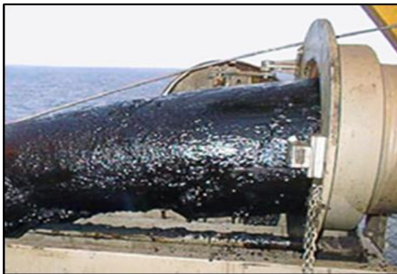
Figure 3. Removing paraffin by pigging Photo by Mokhatab and Towler
