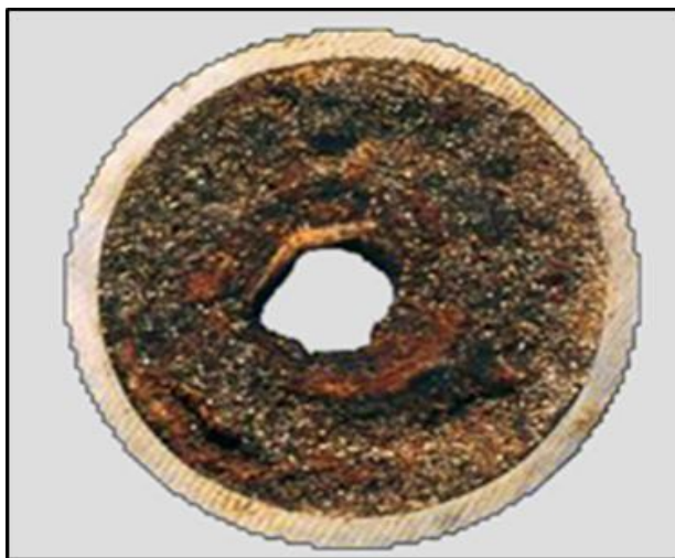
Figure 2. Diameter flow compromised by the deposition of paraffin. Photo by Mokhatab and Towler.
